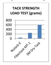
Plywood/18oz/18oz, <u>3M® Dry Tack</u> excellent tack, not repositionable, <u>Fibertack MT-1</u> good tack, repositionable, <u>NuTack-E®</u> low tack, repositionable
